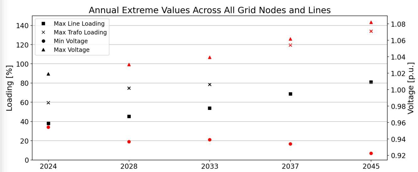
→ Voltage limits are exceeded as early as 2028, well before the transformer overload occurs.
